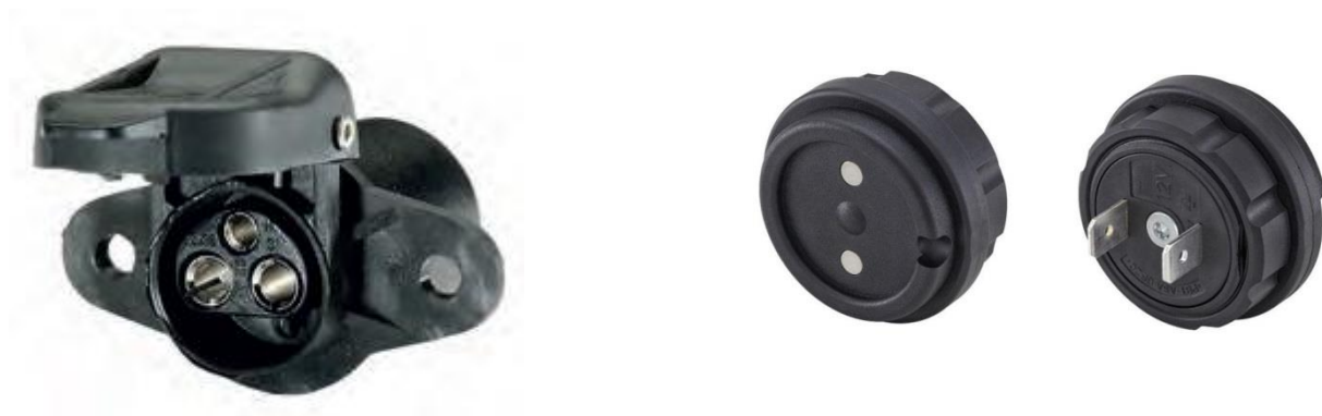
Plastic model, 3-pole, 25A, 2.5 mm 2 (DIN 9680)
